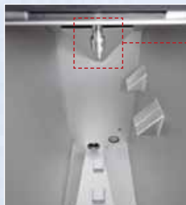
Rotating cleaning nozzle in cockpit recovery tank
