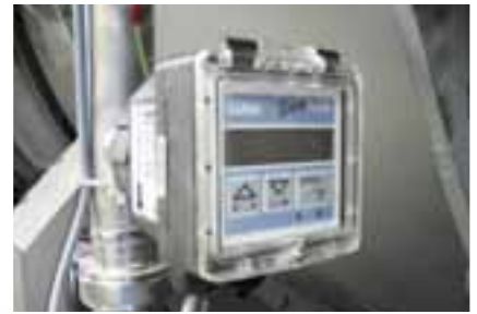
Exact water supplies with inductive-type flowmeters
