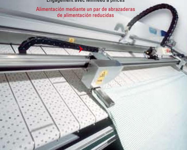
Feeding with extended feed-band table with inbuilt suction
