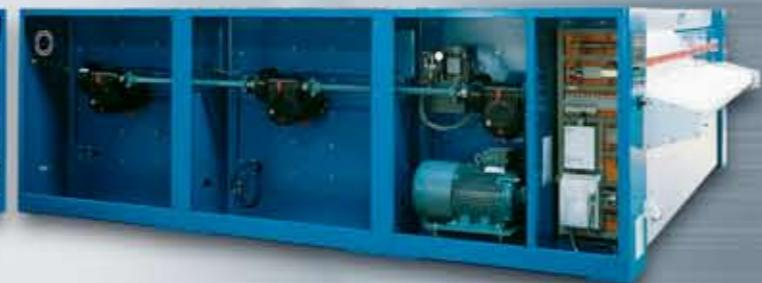
**1** The ironer roll is driven by a frequency-controlled AC motor through a fully enclosed planetary gearbox fitted directly to the roller. The roll is supported by large, heavy-duty SKF roller bearings. The bearings are easily accessible mounted in the ironer side frames which eases maintenance.
