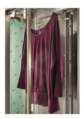
The decisive factor for this stunning finishing quality is the high-pressure water spraying technology. The micro-fine nebulization allows the water to permeate into the fibre and makes it swell. The effect is amazing: Even hard creases, e. g. in linen garments or jeans, disappear. The unwelcome washeffect is also avoided.
