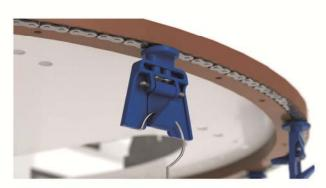
The improved Conveyor System is driven by a maintenancefree chain system. The transport chain is guided in soft curves through sliding guides rather than via sprocket wheels. This method allows the system to work reliably with minimum maintenance.
