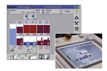
The control systems of the individual modules are connected with the control unit through a BUS cable. Its user-friendly surface allows fast access to all important functions and parameter setting of each module. In addition, programs can be stored and retrieved when necessary.
